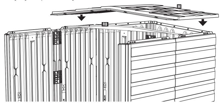
Slightly raise front edge of roof enough to allow positioning of **Roof Brace (RB)** onto the side walls as shown. Lower the roof onto the walls and align **Roof Brace (RB)** into pocket in **Repeat Roof (M)**.
